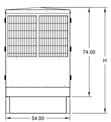
All enclosure models are 200 MPH wind rating certified in accordance with IBC2018 and ASCE/SEI 7-16 standards.
